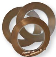
**Copper and Specialty Foils** are used in making your Tiffany style lamps and window panels. The adhesive backed foil is wrapped around each piece of glass to be soldered together. The narrower foil sizes will produce a more delicate lead line and use less solder as well. Each 36 yard long by 1.25 mil thick roll is individually wrapped for long shelf life. Actual size foil widths are shown at right.
